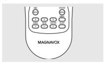
Press the respective buttons on the remote (REAR + -, CENTER + - and SUBW + -) to adjust the output level between -15dB ~ +10dB.
